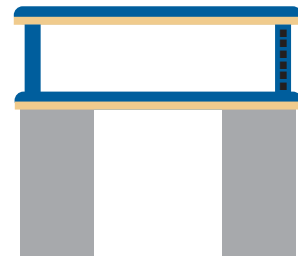
PART NO. INCLUDES TB0602- (2) 16" instrument riser supports (1 with power) 12" deep instru. riser shelf worksta. + shelf back stops
