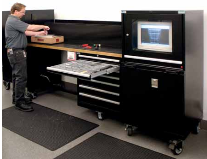
A mobile computer cabinet is paired with a mobile industrial workbench in Toyota Racing Development's machine shop.
