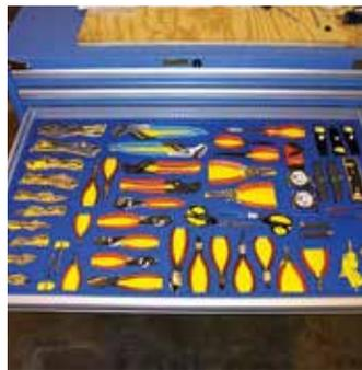
The 5S visual workplace, where tools are easy to find and located right at the work area, leads to a clean, efficient work environment.
