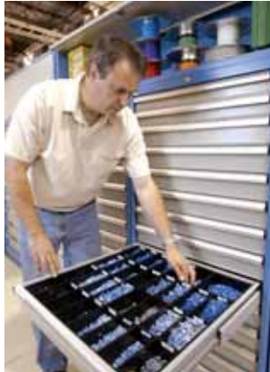
Open shelving (left) is very inefficient at storing small items. High density drawer and shelf storage (right) enables storage of small items in right-sized compartments, increasing cubic capacity and organization.
