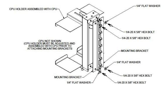
Note: Inner and Outer Channels  $\underline{must}$  be assembled and adjusted to the CPU  $\underline{prior}$  to attaching Mounting Brackets
